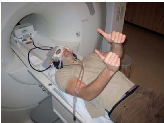
**Fig. 2.** The acquisition setup. The subject's head has been fixed to the scanning table. The mobile transceiver is visible over the subject's right eye.
