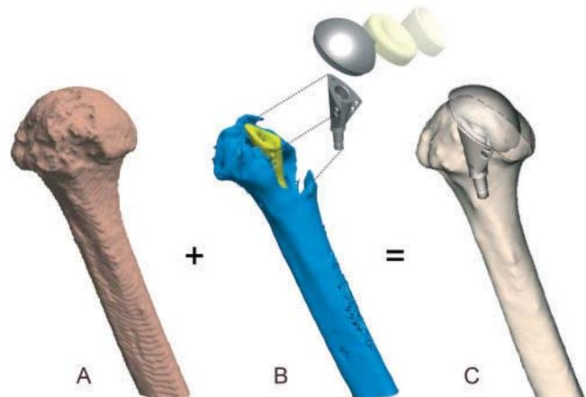
**Fig. 9** Pre-operative surface model A and post-operative surface model B. Scattering caused by the prosthesis prevents complete segmentation of the CT data. However, by overlaying the two scans, the prosthesis position and alignment can be reconstructed to give C. The resulting models were used as input for the ROM simulations
